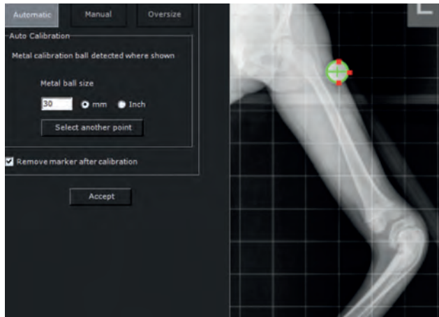
Figure 2.3 Image calibration using a scalar ball.
